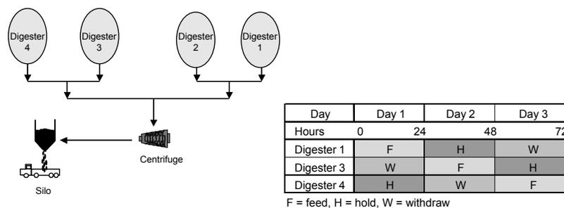
**Figure 1** TITP—Thermophilic anaerobic digestion process and digester cycles for batch operation
