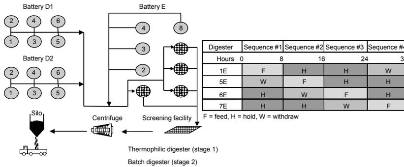
**Figure 2** HTP–Thermophilic anaerobic digestion process and digester cycles for batch operation
