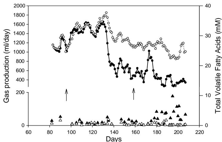
Fig. 1. Effect of DBP and DEHP addition on gas production on volatile fatty acids level. The arrows indicate the beginning (day 86) and end (day 166) of the PAEs addition period. DBP and DEHP were sorbed into the sewage sludge and fed at a load of 12.5 mg/day of each phthalate. (—●—) gas (test digester); (----○----) gas (control digester); (▲) VFAs (test digester); and (△) VFAs (control digester).
