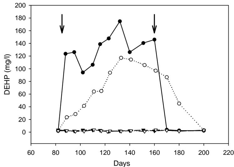
Fig. 4. DEHP concentrations in digesters. Arrows indicate the 12-weeks period with PAEs addition. (—●—) influent test digester; (---○---) effluent test digester; (—▼—) influent control digester; and (---▽---) effluent control digester.
