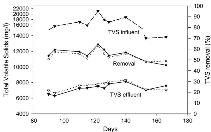
Fig. 2. Total volatile solids in influents and effluents and TVS removal during the 12-weeks PAEs addition period. Solid symbols: test digester; and open symbols: control digester.
