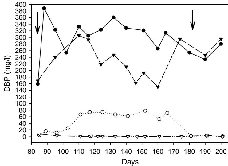
Fig. 3. DBP concentrations in digesters. Arrows indicate the 12-weeks period with PAEs addition. (—●—) influent test digester; (---○---) effluent test digester; (—▼—) influent control digester; and (—▽—) effluent control digester.
