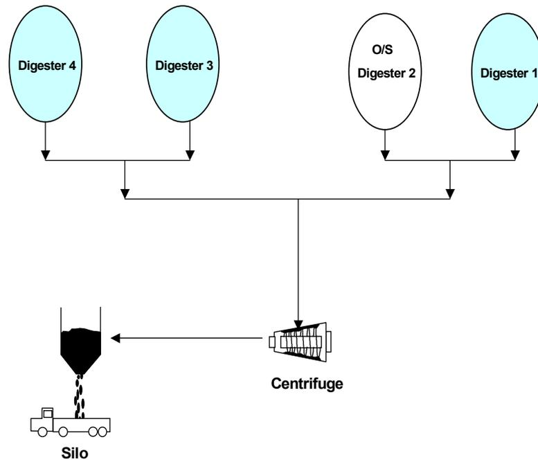
**Figure 1b. TITP-Digester cycles for batch operation**
