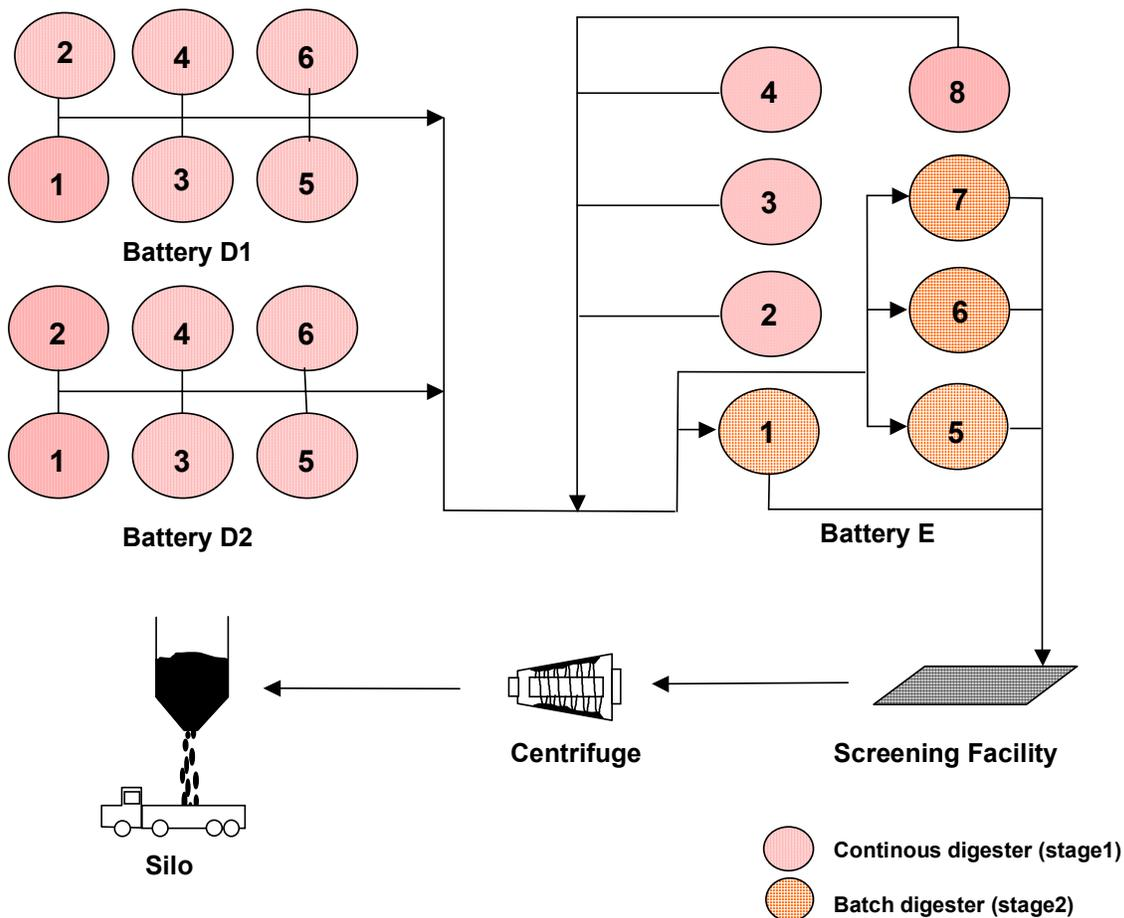
Figure 2b. HTP- Digester cycles for batch operation
