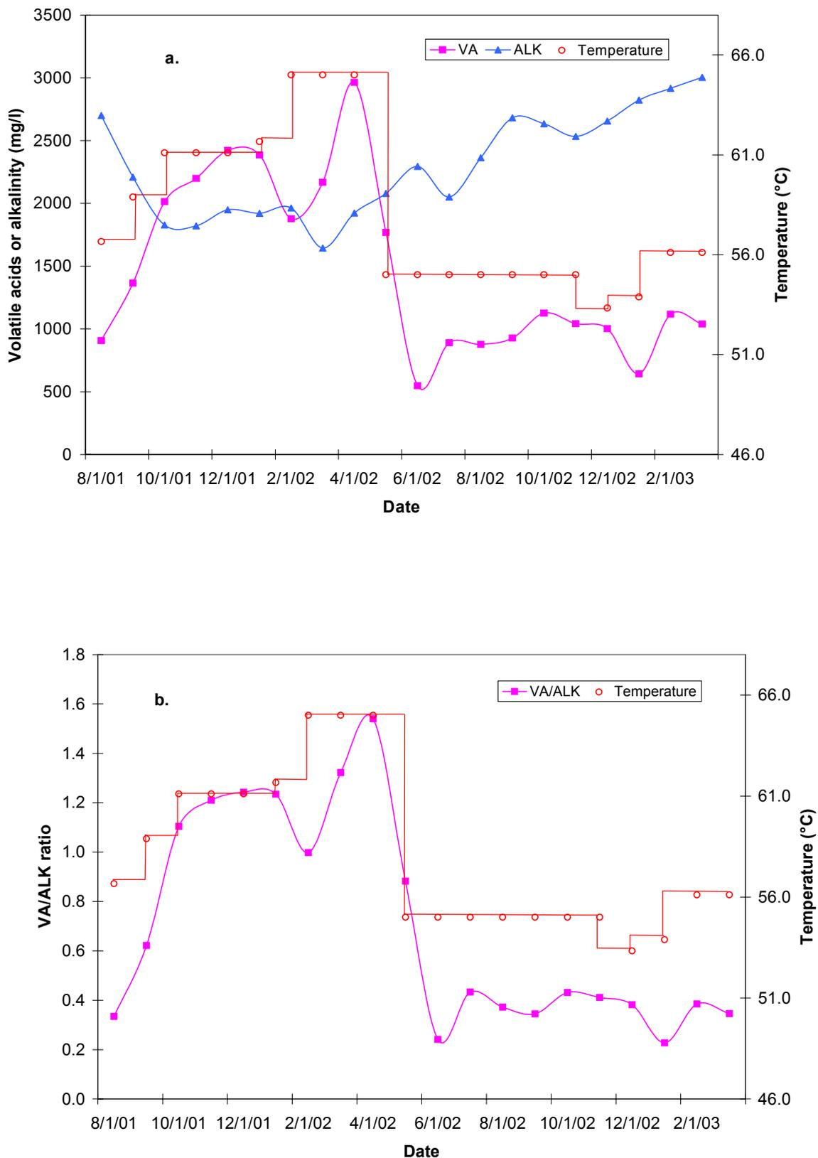
**Figure 13. HTP Pilot - Volatile solid destruction versus digester temperature**
