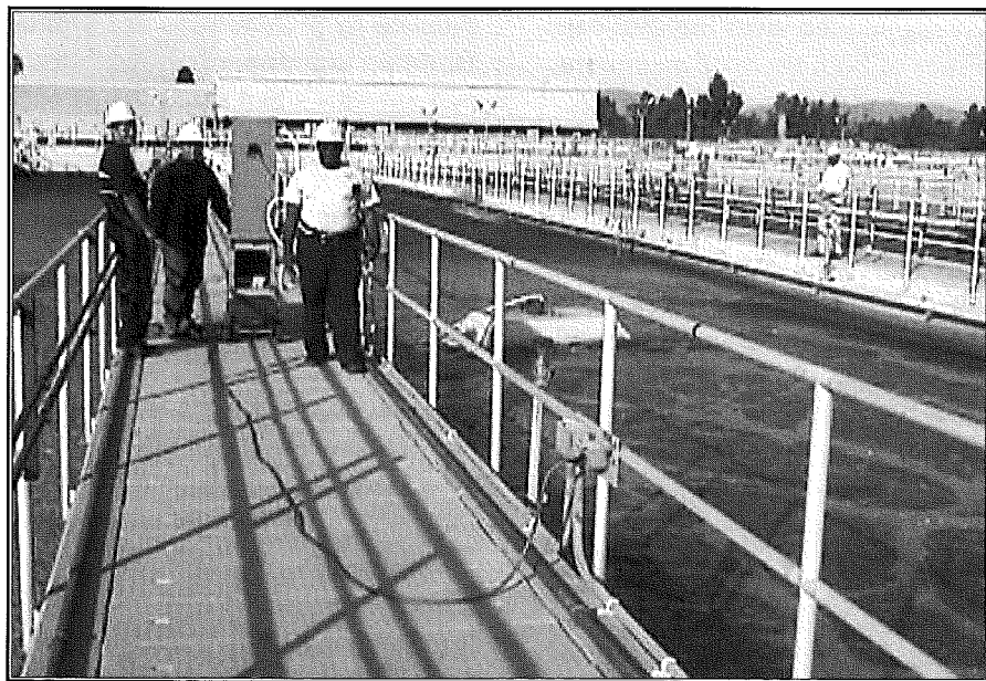
Oxygen transfer efficiency testing at the D. C. Tillman Water Reclamation Plant. Shown on a walkway dividing two aeration tanks are Miguel Zermeno, Alfredo Magallanes and Cornelius Reffegge testing oxygen transfer efficiency at an aeration basin. On the far walkway (right) Dipak Patel takes water temperatures.
