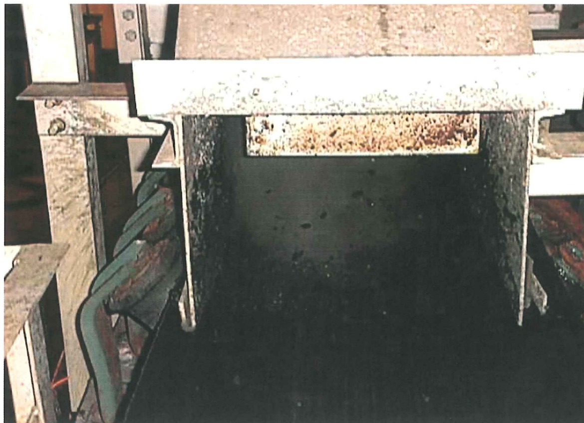
(f) Wet cake from centrifuges to conveyor belts.
